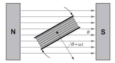
The coil rotates 50 times per second in a field of flux density 0.215 T. The coil has 2650 turns and cross-sectional area  $2.35 \times 10^{-3} \,\mathrm{m}^2$ . (Note that  $\theta$  = 0 when t = 0)
