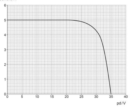
The solar panel has a surface area of 1.2 m<sup>2</sup>. Determine the efficiency of the solar panel when it is operating at its maximum power output. [4]
