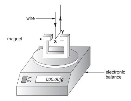
The part **XY** of the wire which is in the magnetic field, has been placed carefully so that the current is from front to back at 90° to the direction of the magnetic field. When there is no current the balance is reset to display 000.00 g. When there is a current in the direction shown, the magnetic force results in a positive reading on the display of the balance. However, this signifies an upward force on the wire.
